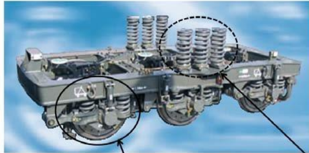
Primary Suspension between axle and bogie Secondary Suspension between bogie and car-body frame
